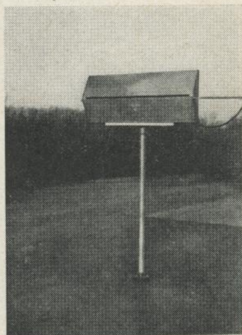
FIG. 18A—Photograph of Chrysler building 4—element UHF television array. FIG. 18B—One element of the Chrysler building television array set up for test.
